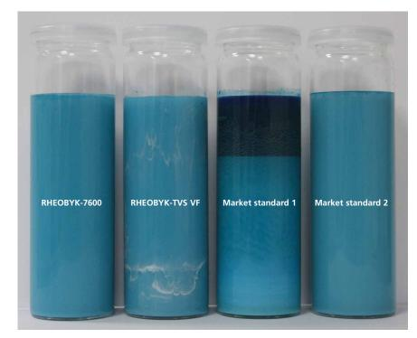
Test system: Pure acrylic, PVC 19 % Dosage: 0.1 % active substance based on
