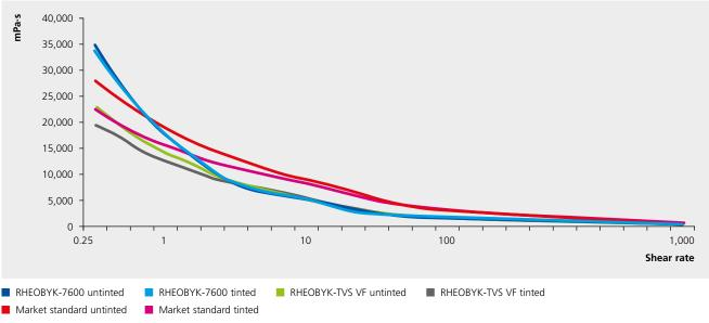
Test system: Pure acrylate, PVC 19 %
